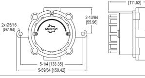
The **Model 862E Explosion-Proof, Heavy-Duty Thermostat** is designed for hazardous-location temperature control of heating, cooling, or ventilation systems and features an adjustable set point knob for easy and convenient set point adjustment.
