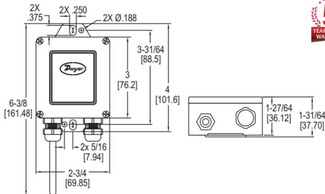
The **Series O-4 Outside Air Temperature Sensor** is great for monitoring ambient air temperatures in outdoor applications. The temperature sensors are mounted in a NEMA 4X enclosure with integral mounting tabs.
