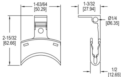
The **Series CC1 Averaging Temperature Sensor Clips** are used to mount the capillary of an averaging temperature sensor to the wall of the duct or air handler. Slots are provided for using nylon zip ties to hold the tubing in place, if needed.
