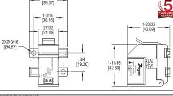
The **Model MSCS Miniature Current Switches** are low cost solutions for monitoring on and off status of light to medium current loads in compact spaces. This unit has a split core design and has a fixed set point of 0.15 amps. It is designed to detect changes in operating current to prevent motor belt loss, slippage, or mechanical failure.
