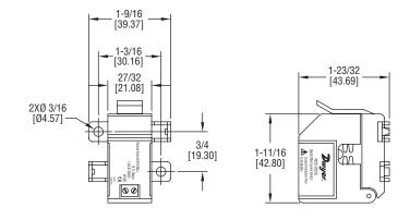
The **Model MSCS Miniature Current Switch** is a low cost solution for monitoring on and off status of light to medium current loads in compact spaces. This unit has a split core design and has a fixed set point of 0.15 amps. It is designed to detect changes in operating current to prevent motor belt loss, slippage, or mechanical failure.
