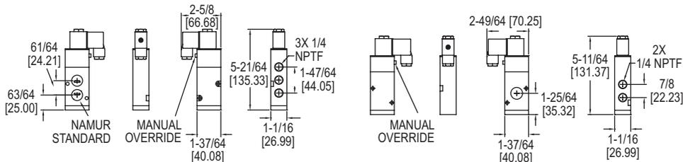
The **Series SN Namur Mount Solenoid Valve** is designed to easily mount directly to pneumatic valve actuators reducing the need for tubing, fittings or brackets, thereby reducing assembly cost. The SN solenoid comes with nitrile o-rings and offers a manual override as a standard feature. The 3/2 solenoids are designed for spring return actuators and 5/2 solenoids are designed to be used with double acting actuators. The SN series is available in a variety of voltages for any application.
