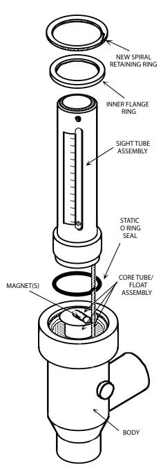
FIGURE 2: PARTIALLY EXPLODED DRAWING OF SERIES SSM ALL METAL FLOWMETERS
