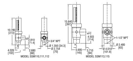
**Series SSM 31 All Metal Flowmeters** are ideal for dirty or opaque fluids, high temperature and high pressure service and harsh environments. The direct reading scale provides ±2% accuracy. Flowmeters can quickly be disassembled without removing the body from the pipeline for easy cleaning.
