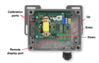
Figure 6: Button board inside of housing
