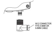
Figure 2: Diagram of M12 connector
