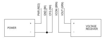
Figure 3: 5 V output wiring
