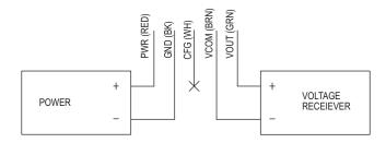
Figure 2: 10 V output wiring
