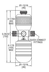
**The Model HP Hand Pump** provides a dual source of pneumatic pressure and vacuum for verifying the calibration of pressure instrumentation. Pump can generate pressures up to 45 psi (3 bar) and vacuum to -27" Hg (-910 mbar). The compact pump is designed for portability and single hand operation.
