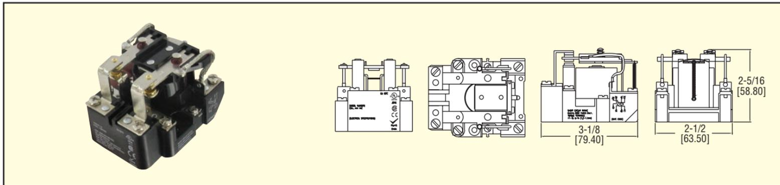
The Series 199 Open Style Power Relays are designed for high AC and DC current applications up to 40 Amps. These mercury-free DPDT relays are available in a variety of trigger voltages and coil resistances to fit most common applications. The riveted housing construction increases the durability and reduces the effects of vibration on the relay.
