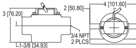
The **Series SFI-100T Sight Flow Indicator/Transmitter** is a low cost and durable flow transmitter that combines our popular 100 Series Sight Flow Indicator with our A-711T output sensor for visual and remote monitoring of flow. The A-711T output sensor has two pulsed voltage signals with one providing a 5 VDC pulse, the other a pulse of the input supply voltage used, ranging from 8-28 VDC and a pulsed output with a frequency change proportional to the flow rate.
