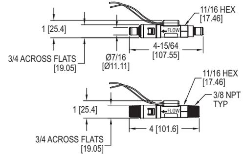
The **Series P3 Polypropylene Flow Switches** fit almost any piping requirements with compatible liquids. Choose the inlet and outlet port to be 3/8" male NPT or 1/4" male "Quick Disconnect" then select a quick disconnect acetal adapter for straight through flow or with a shut off valve.
