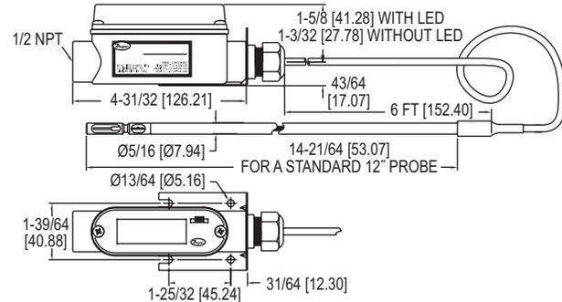
The **Series 641RM Air Velocity Transmitter with Remote Probe** features the same highly accurate heated mass flow sensor as the Series 641, with a remote probe construction. The units 6' cable which connects the sensing probe with the electronic enclosure allows the enclosure to be mounted where it can be more easily accessed.
