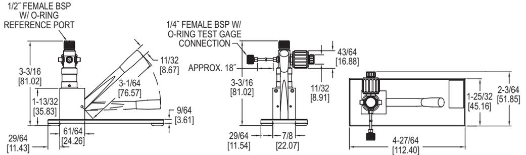
The **Series BCHP Low Pressure Calibration Pump** is able to generate pressure and vacuum for adjusting or calibrating pressure gages, transmitters, or switches. The pump is hand operated and has a pneumatic pressure range of -28 to 870 psi (-0.95 to 60 bar).
