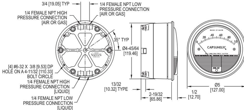
The **Series 4000 Capsuhelic® Differential Pressure Gage** is designed to give fast, accurate indication of differential pressures. The gage may be used as a readout device when measuring flowing fluids, pressure drop across filters, liquid levels in storage tanks and many other applications involving pressure, vacuum or differential pressure.
